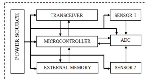
Fig 1. Sensor node architecture
